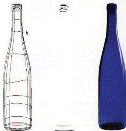
The finished blue bottle mesh in outline, hidden, and in Preview with details on a layer above
